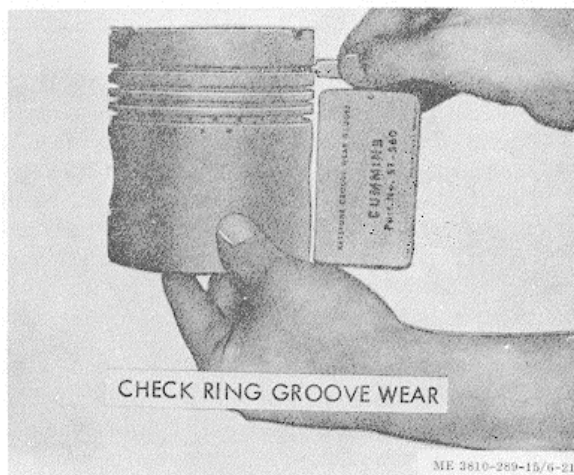
Figure 3-205. Ring groove wear check.
