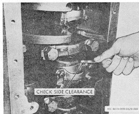
Figure 3-215. Rod-to-crankshaft side clearance check.
